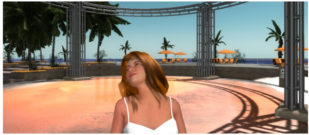
Figure 2. Welcome Area in Blue Mars 3D world (1.51 M triangles @ 30 FPS). The avatar head is tilted back and sideways, copying user head pose. Tracking has no impact on FPS in this scene.
